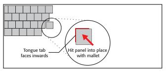
Do not directly hit the edge of the **GenieMat FF** tiles with a mallet or hammer. Use a wood block flush with the edge to distribute the load and protect the edges as the tiles are hit into place.
