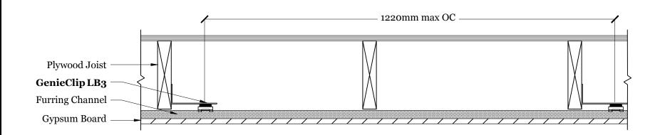
Note: Minimum of 3mm spacing between Plywood Joist and Furring Channel
